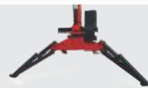
Robust stabilizer legs ensure a stable setting even on an uneven work terrain.
