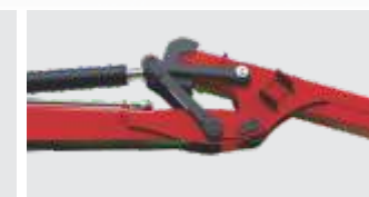
A four-joint "K" mechanism on the restraint between the lifting and the swinging arm provides for excellent work characteristics of the crane.
