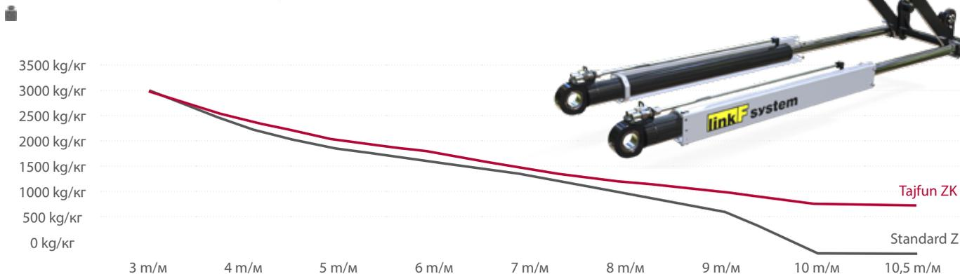
🇩🇰 The new »linkF system« solution significantly increases the power of the crane in the extended position compared to conventional Z-cranes. The innovative joint mechanism between the booms provides 20% more lifting power with the lever mechanism in the extended position, which enables the easier and faster loading and unloading of cargo and increases work productivity. In the variant with two telescopic booms, the crane can cover a working area of up to 10.5 m.
