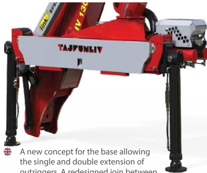
A new concept for the base allowing the single and double extension of outriggers. A redesigned joint between the central part of the base and the bridge – fewer critical points.
