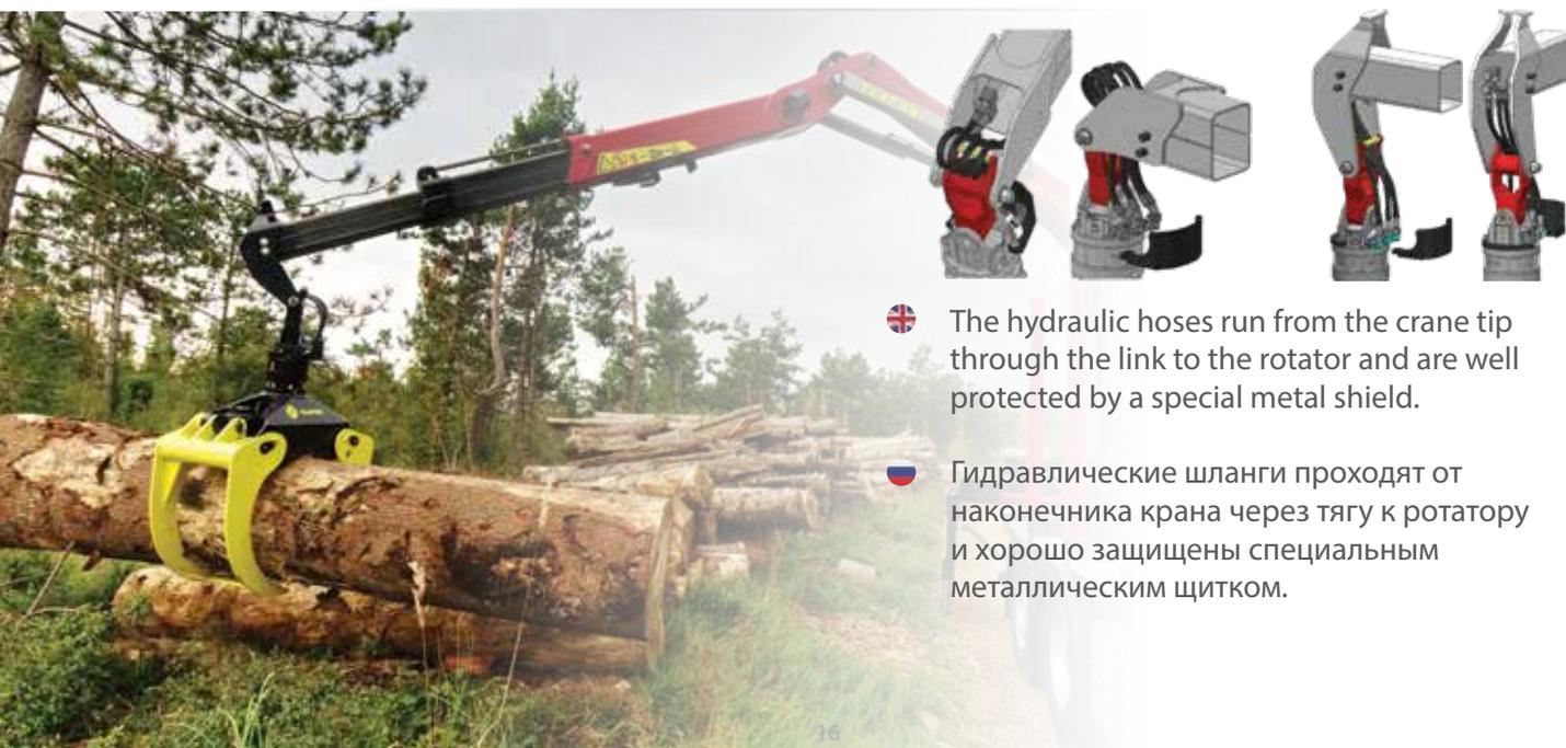
🇬🇧 The hydraulic hoses run from the crane tip through the link to the rotator and are well protected by a special metal shield.
