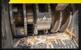
The wood chipper is entirely made of Hardox, featuring an extremely robust rotor and wide knives, ensuring a cleaner cut and less dust even when processing small material and logging residues. Its compact design, without unnecessary covers, allows for easy maintenance and long-lasting reliability.
