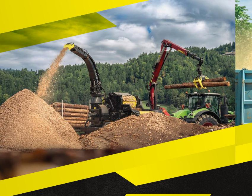
The automatic feed and slow-rotating rotor with optimized technology ensure uniform, clean, high-quality chips with minimal dust.
